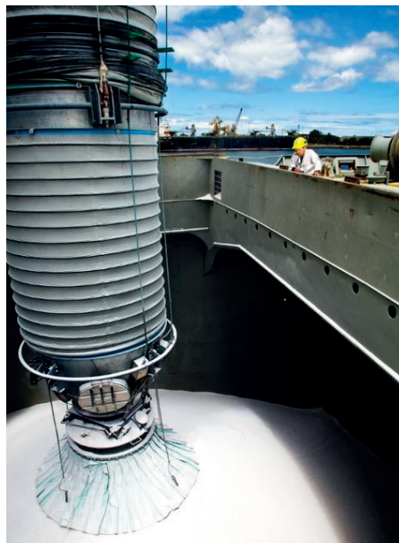
Fig 2. Alumina being loaded at Alcoa's berth at the Bunbury Port for export from Western Australia. (This photograph was provided courtesy of the Australian Aluminium Council.)
